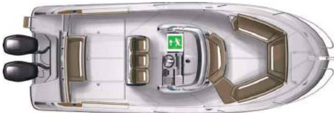
Emergency exits in case of fire - Companionway
