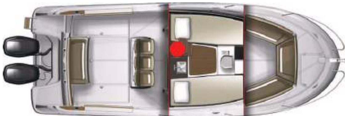
Position of portable extinguishers (not supplied)
