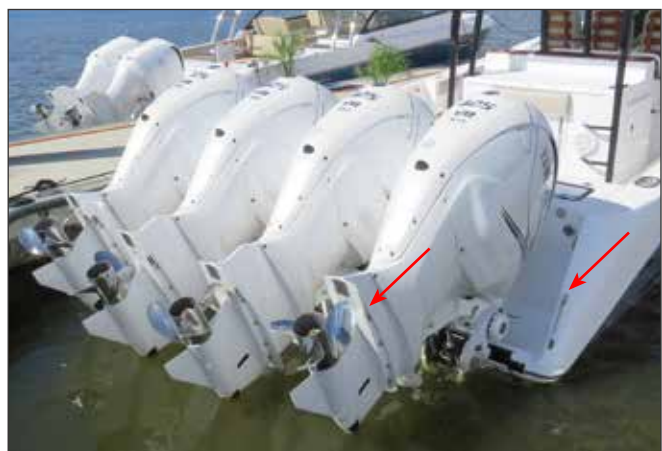
Stern Grab Rail & Anti-Ventilation Plate for Unassisted Boarding Situations
