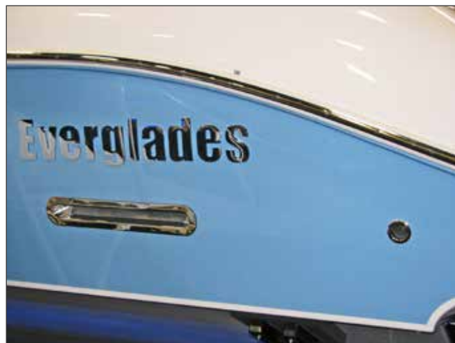
Scupper Drain Thru-hull Fittings
