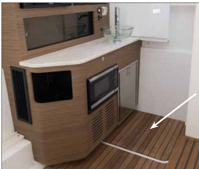
Removable Cabin Floor Panel Remove To Access Forward Bilge Pump & Drain Sump Pump
