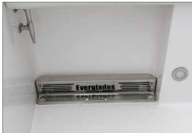
Typical Scupper Drains & Drain Rail
