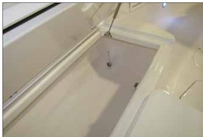
Bow Storage Compartment Drain & Drain Plug
