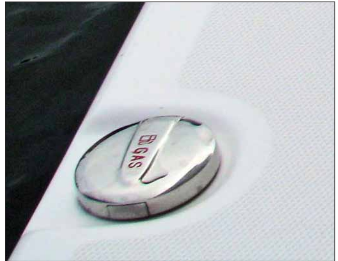
Typical Fuel Fill
