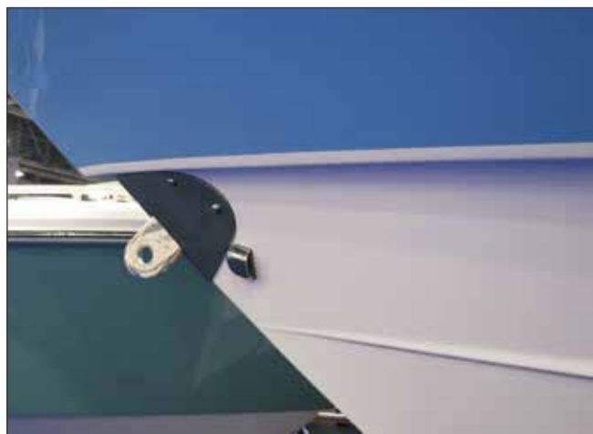
Rope Locker Drain Fitting in Hull Side
