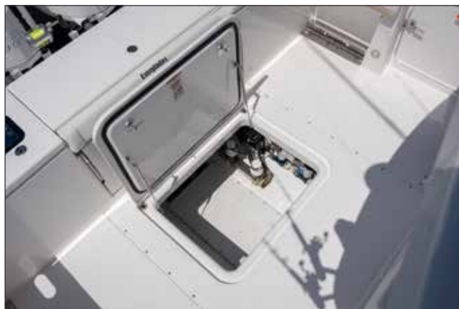
Mechanical Systems Compartment Hatch
