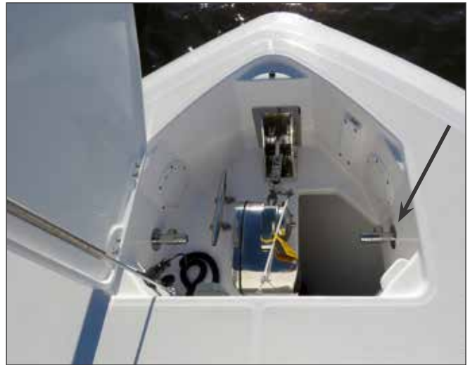
Fresh Water Washdown Faucet in Winch Compartment
