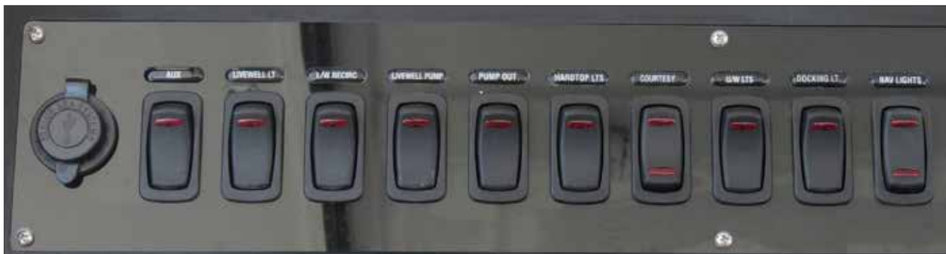
Port Helm Accessory Switch Panel
