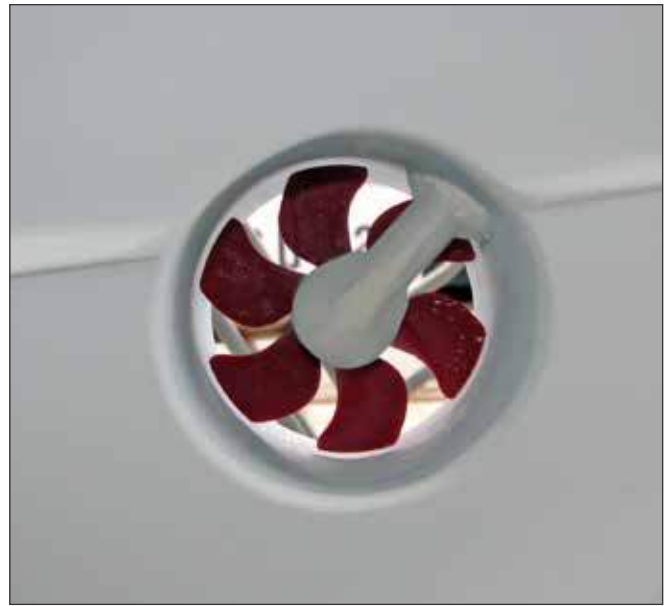
Typical Bow Thruster Drive Unit, propeller & tunnel
