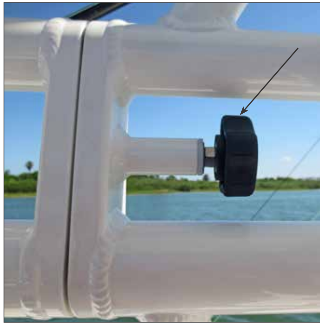
Hand Bolt On Each Side Securing Upper Station Sections
