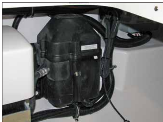
Power Steering Unit in the Systems Compartment
