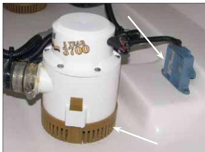
Bilge Pump Strainer and Automatic Switch
