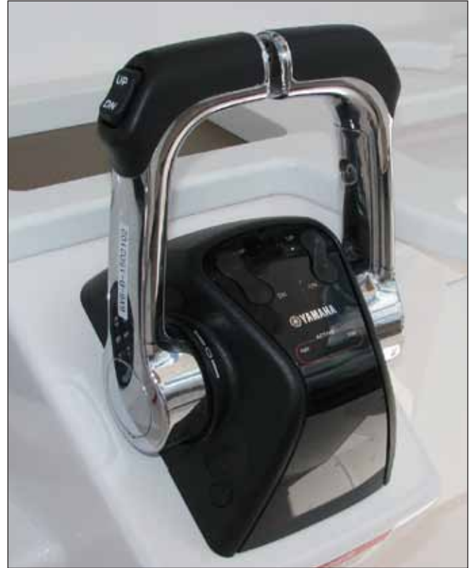
Typical Yamaha Twin Engine Electronic Controls
