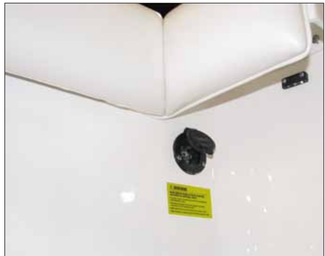
Shore Power Inlet Connection
