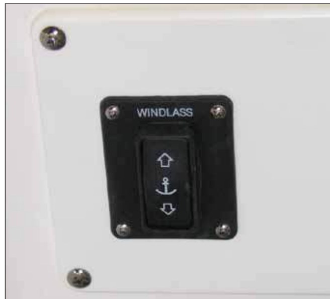
Windlass Switch in Rope Locker Near Windlass
