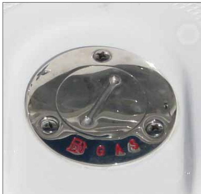
Typical Fuel Fill
