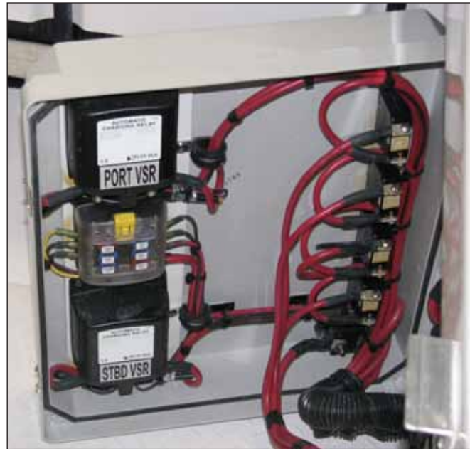
Battery Switches, Emergency Parallel Switches, PT & STBD Voltage Sensitive Relays, Main Circuit Breakers and Continuous Power Fuse Panel
