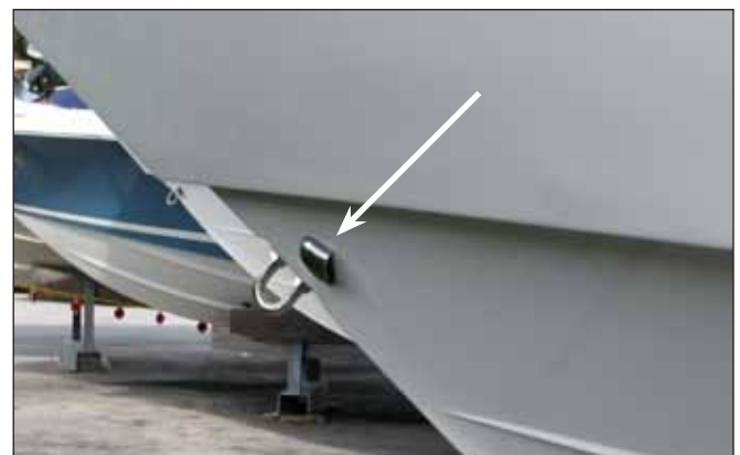
Rope Locker Drain Fitting in Hull Side
