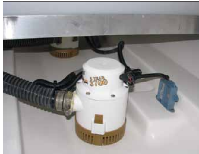
Typical Bilge Pump and Automatic Switch
