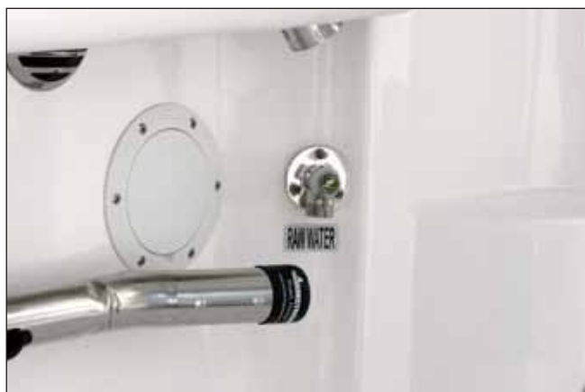
Typical Washdown Hose Connection
