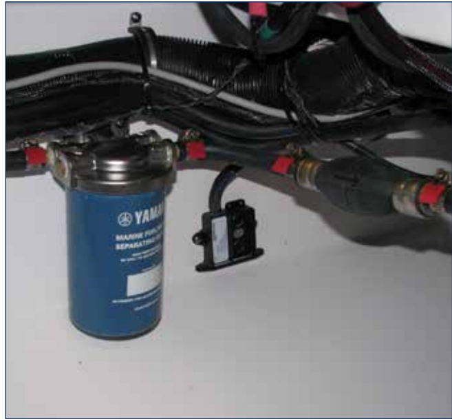
Typical Yamaha Fuel Filter In Aft Systems Compartment
