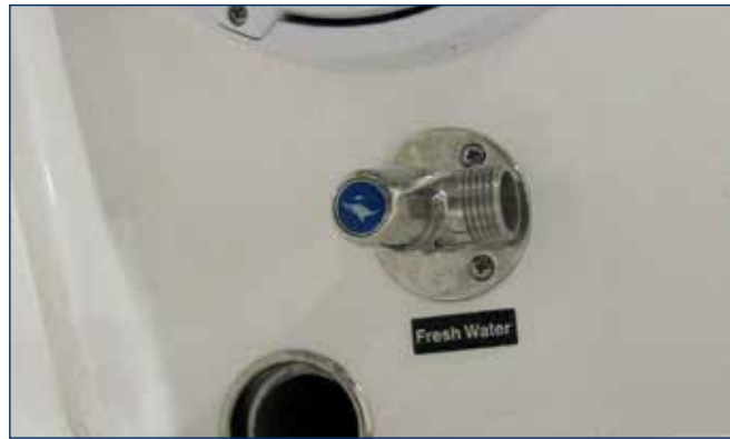
Fresh Water Washdown Hose Connection
