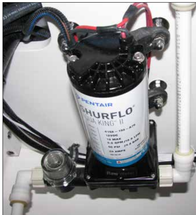
Raw Water Pressure Pump & Sea Strainer
