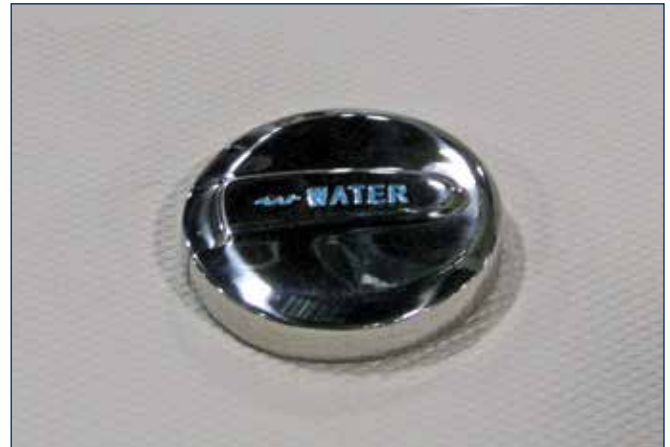
Fresh Water Fill
