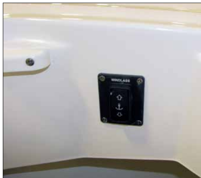
Anchor/Rope Locker Windlass Switch
