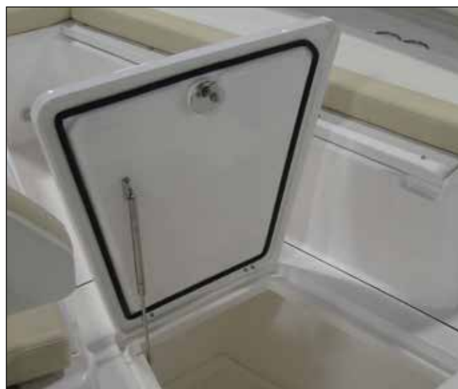
Hatch Twist Lock Latch & Gas Charged Spring
