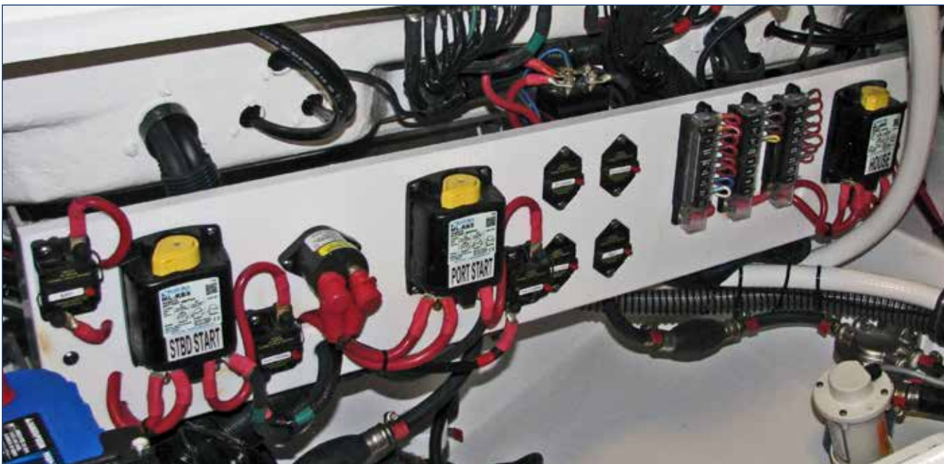
Battery Switches, Fuse Panels & Main Circuit Breakers - Twin Engine Models
