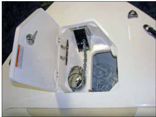
Windlass & Rope Locker
