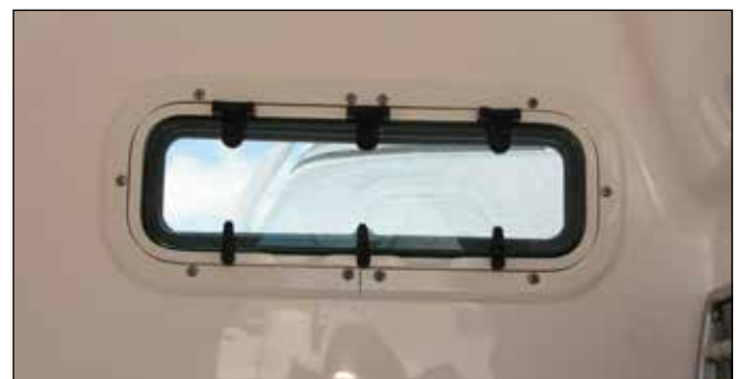
Cabin Port Window & Twist Action Locks
