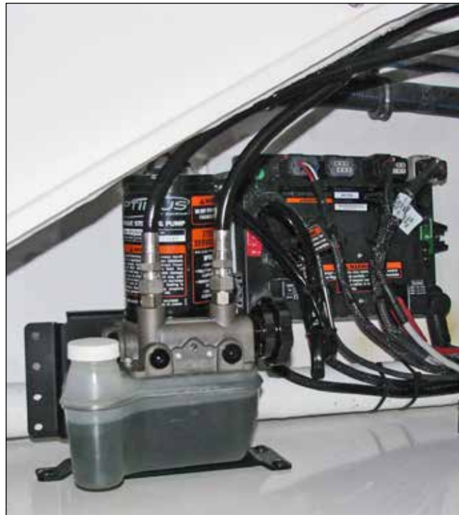
Typical Electronronic Steering Unit
