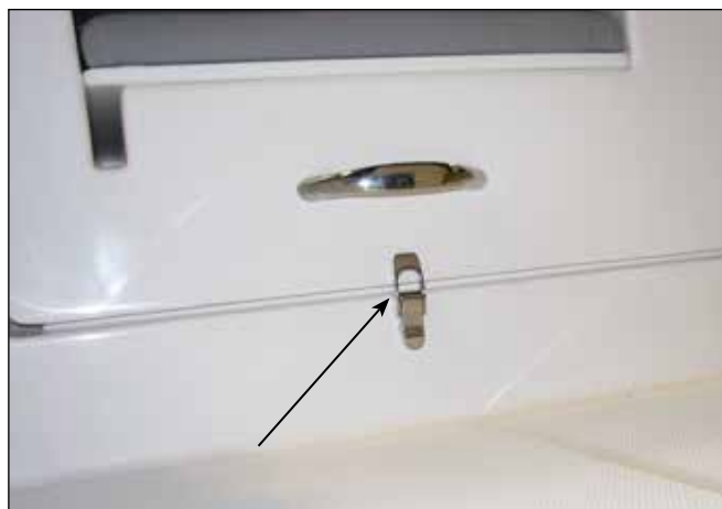
Stern Seat Base Cam Action Compression Latch
