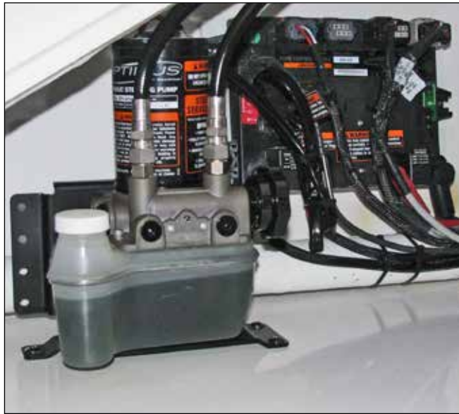
Yamaha Electronic Steering Pump & Control Panel
