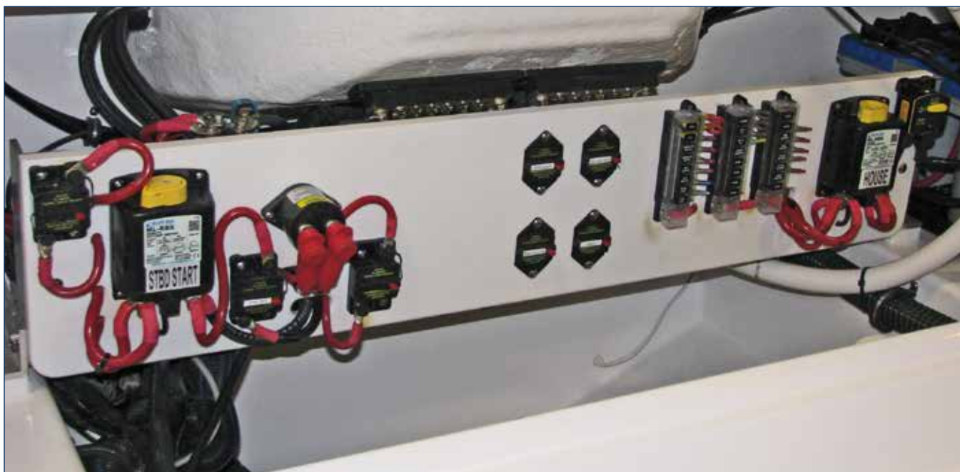
Battery Switches, Fuse Panels & Main Circuit Breakers - Single Engine Models
