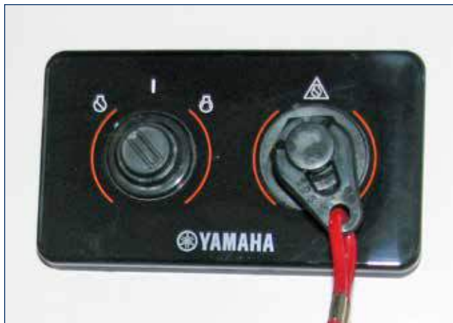
Typical Single Engine Yamaha Command Link Ignition
