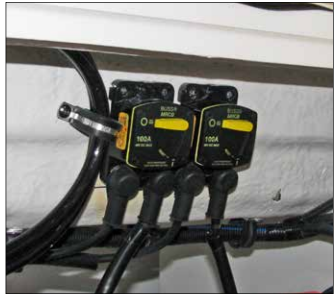
Typical Yamaha Engine Charging Circuit Protection
