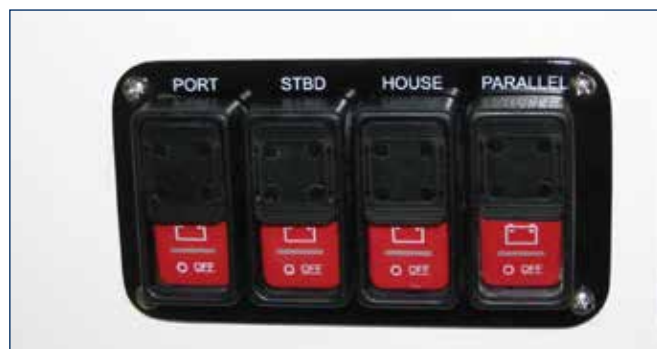
Twin Engine Remote Battery Switches
