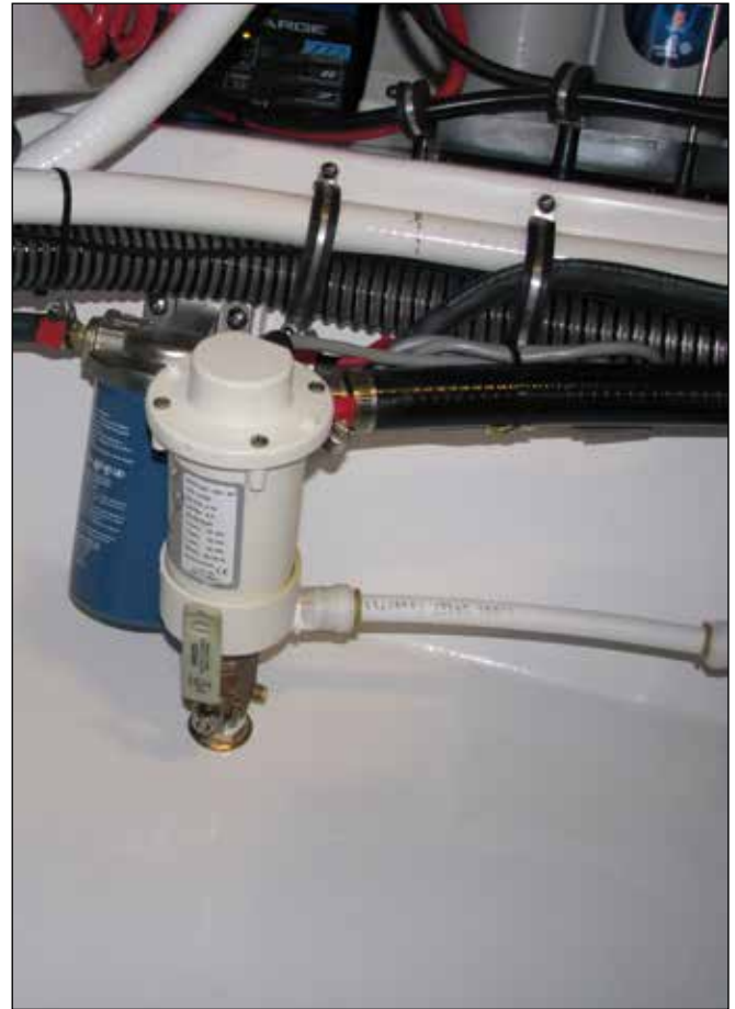
Baitwell Supply Pump & Seacock
