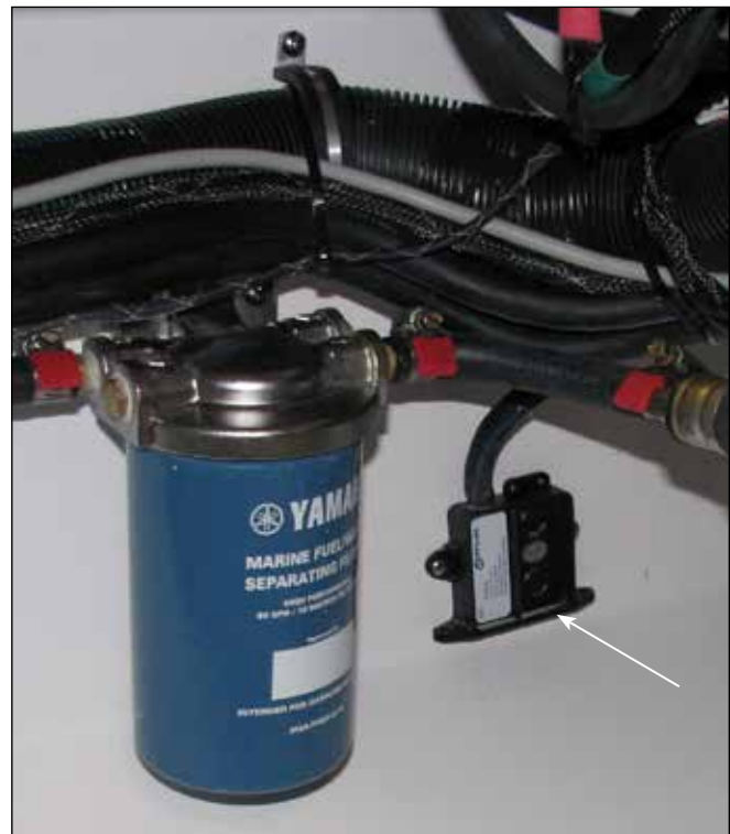
Bilge High Water Alarm Automatic Switch
