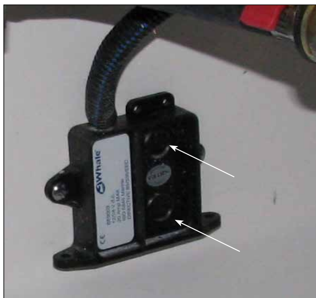
Bilge High Water Alarm Automatic Switch Recessed Test Discs
