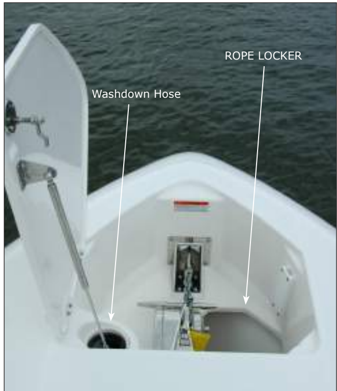
325 Center Console Anchor/Windlass Compartment
