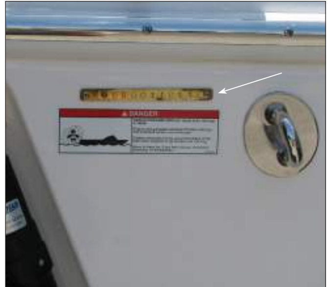
Hull ID # On Starboard Side of Transom
