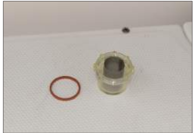
Typical Fresh Water Pump Strainer Removed for Cleaning
