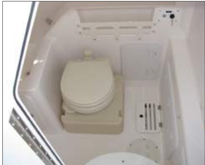
Marine Toilet and Holding Tank
