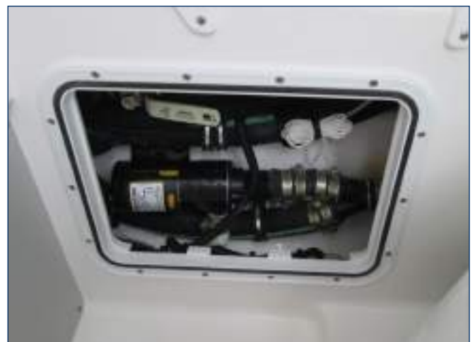
Macerator Access Hatch
