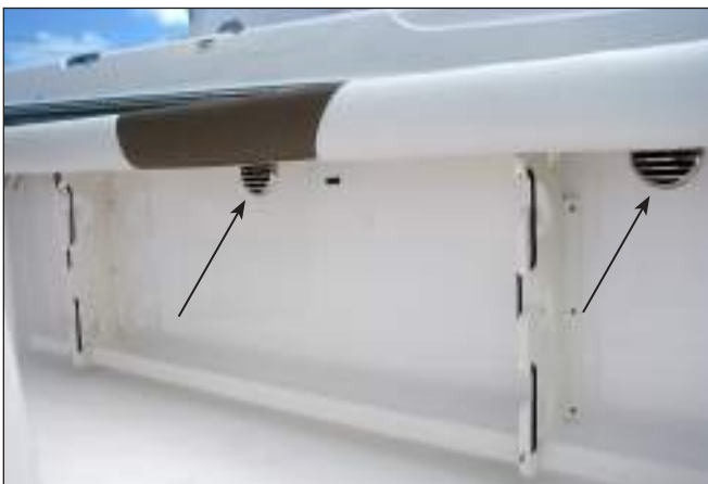
Bilge Vents in the Side of the Cockpit Liner
