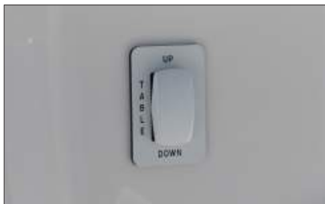
325 Center Console Table Pedestal Control Switch
