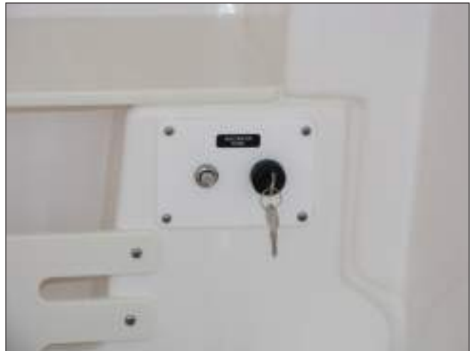
Waste System Pump Out Switch Panel
