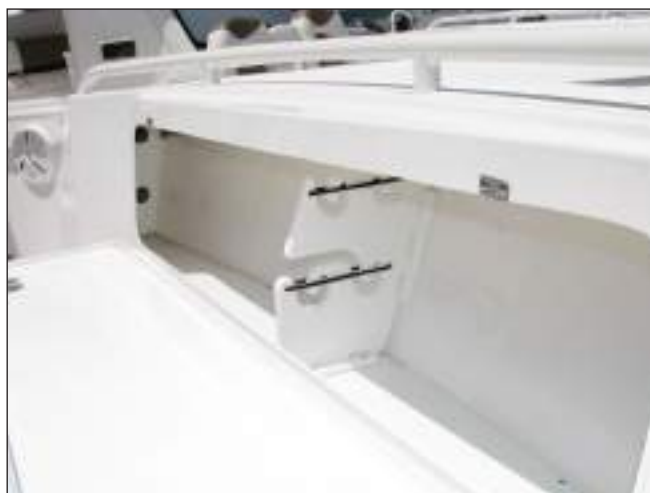
Typical Rod Locker at Bow
