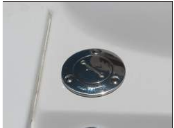
Fresh Water Fill
