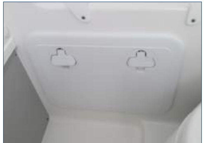
Macerator Access Hatch
