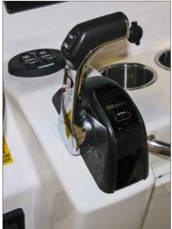
Typical Yamaha Single Engine Electronic Control
