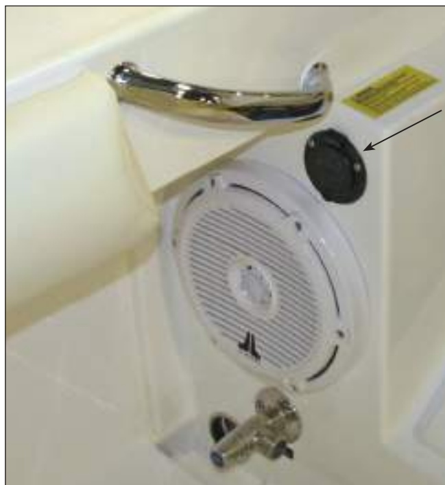
Typical 120 Volt Shore Power Inlet Connection
