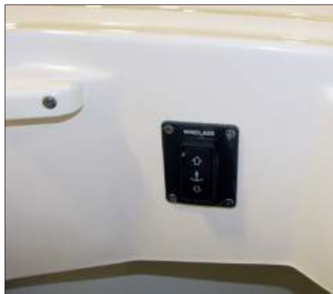
Anchor/Rope Locker Windlass Switch
