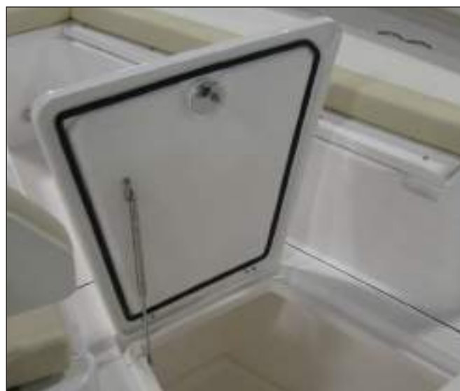
Hatch Twist Lock Latch & Gas Charged Spring
