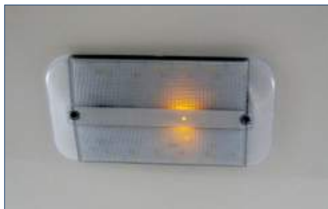
Aft System Compartment Light
