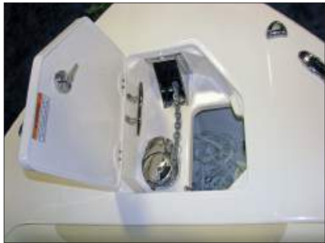
Windlass & Rope Locker
