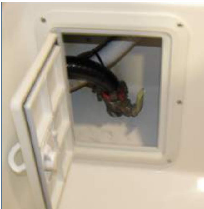
Forward Bilge Access Door
