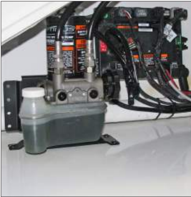
Typical Yamaha Electronic Steering Pump & Control Panel
