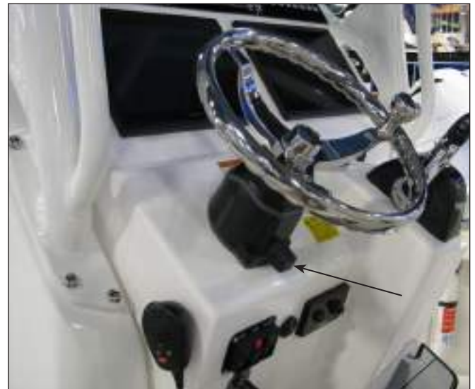
Typical Tilt Steering Wheel & Tilt Lock Lever
