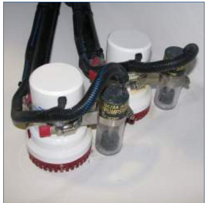
Aft Bilge Pumps & Automatic Switches
