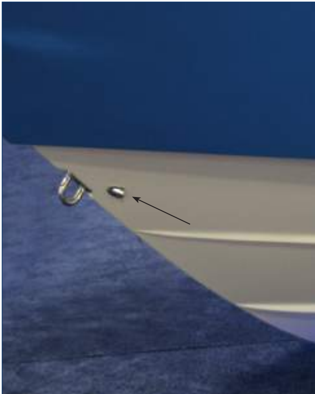
Rope Locker Drain
