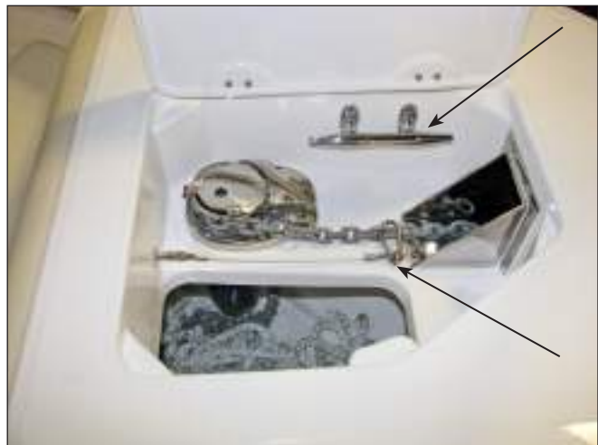
Windlass Chain Binder & Anchor Line Cleat
