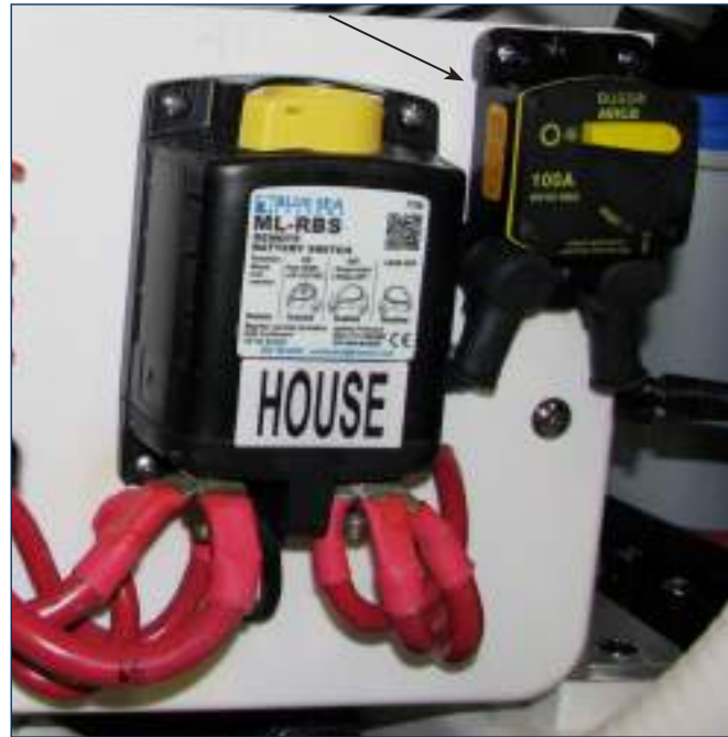
Typical Yamaha Engine Charging Circuit Protection
