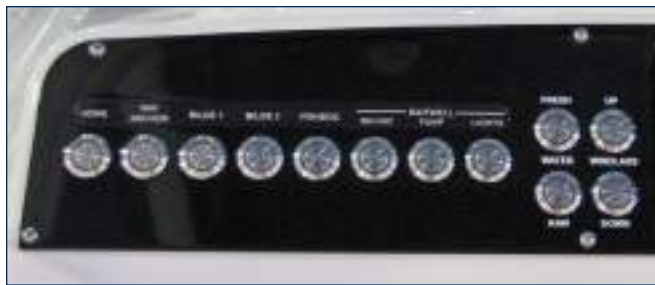
Port Side Helm Switches
