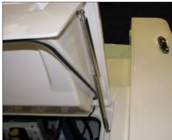
Stern Seat Base Gas Charged Spring & Support Strut
