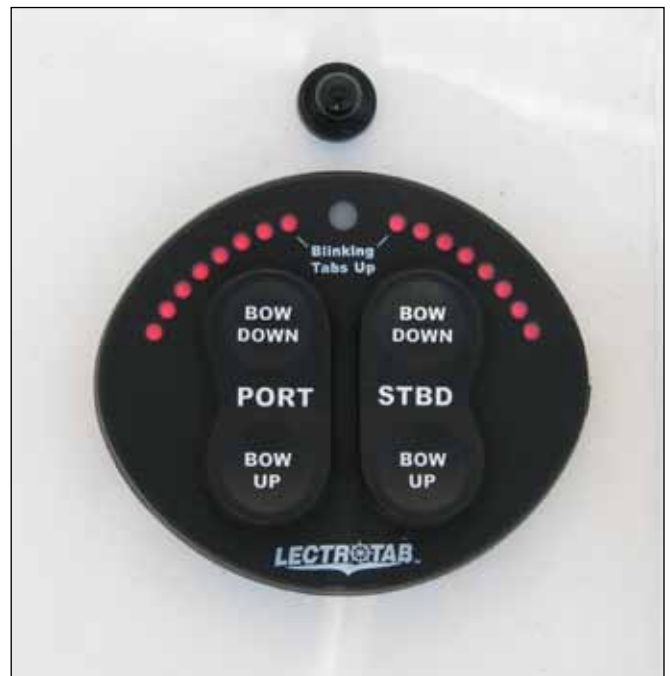
Optional LED Indicator Trim Tab Switch
