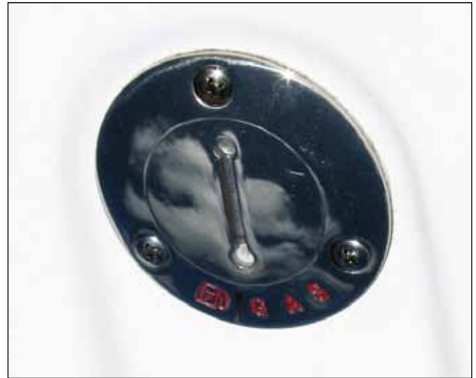
Typical Fuel Fill
