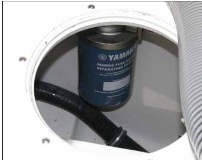
Fuel Filter Below Splashwell
