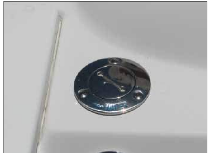
Fresh Water Fill
