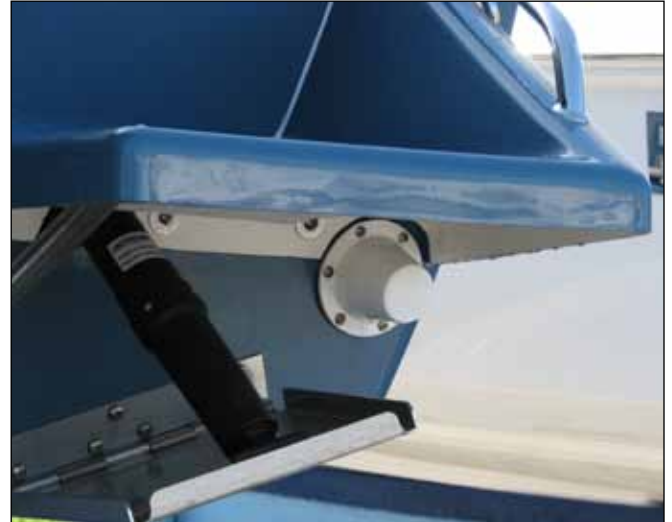
Scupper Drain Check Valve Assembly
