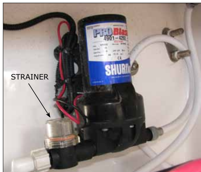
Typical Fresh Water Pump and Strainer
