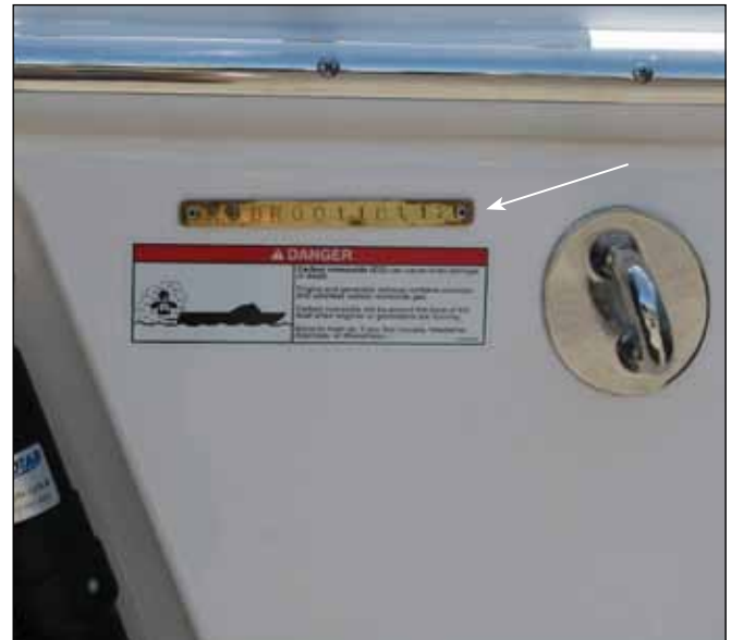
Hull ID # On Starboard Side of Transom
