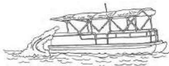
FIGURE 1.5 EXHAUST ACCUMULATION DUE TO HIGH BOW ANGLE OR SLOW SPEED
