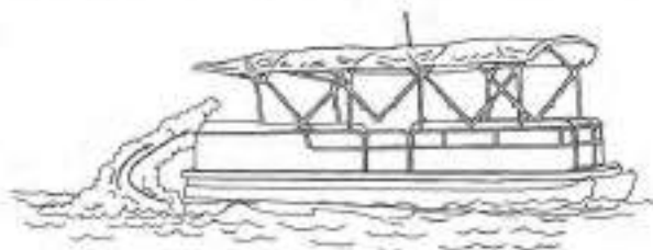
FIGURE 1.4 EXHAUST ACCUMULATION WHILE CANVAS IS IN PLACE
