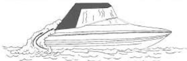
FIGURE 1.4 EXHAUST ACCUMULATION WHILE CANVAS IS IN PLACE
