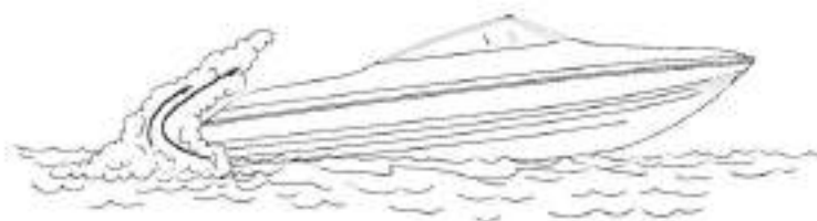
FIGURE 1.5 EXHAUST ACCUMULATION DUE TO HIGH BOW ANGLE OR SLOW SPEED
