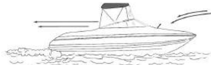
FIGURE 1.6 DESIRED VENTILATION THROUGH THE BOAT
