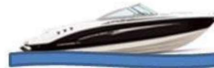
Incorrect Causes boat to "porpoise"
