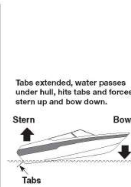
Figure 3.7 Trim Tab Operation
