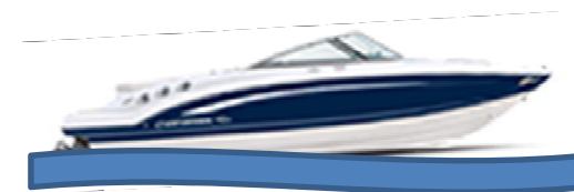
Incorrect Causes boat to "porpoise"
