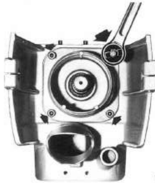
12 - loosen the four screws securing the clutch shaft bearing housing and pry it out using two screw drivers (13).
