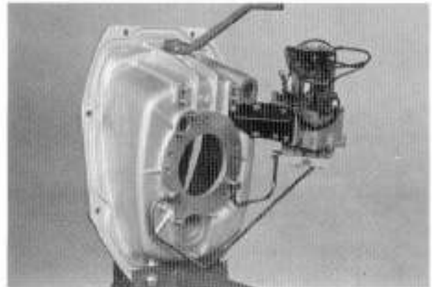
Hydraulic Control Lines Installed
