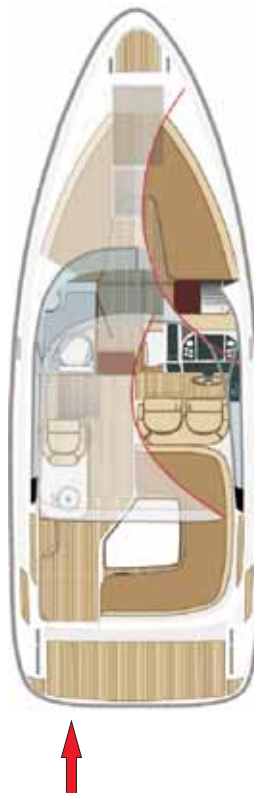
Figure 8. Location of working decks and reboarding ladders.
