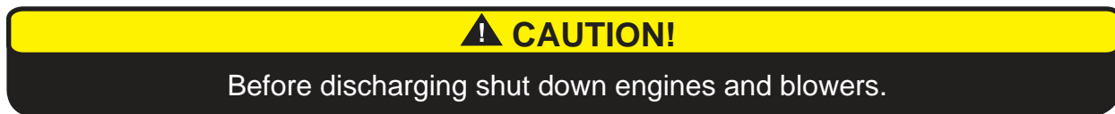
Figure 4. A warning plate about shutting down engine and blowers before discharging the fixed extinguishing system.
