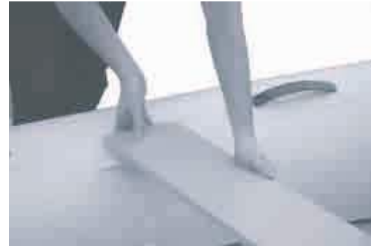
THE REMOVABLE SEAT IS EASIER TO FIT IF THE BOUYANCY CHAMBER IS SLIGHTLY DEFLATED
